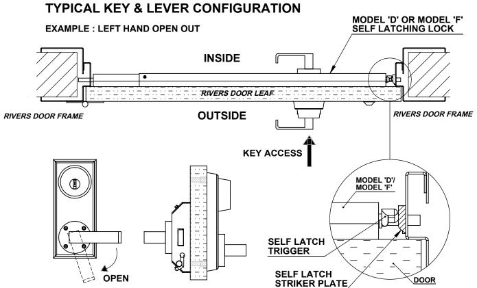
KEY & LEVER - EXTERNAL ACCESS TO MODEL 'D' & MODEL 'F' SELF LATCHING LOCKS
